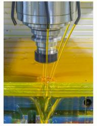
High precision machining requires highest filtration efficiency of coolants. Micro filtrated coolants contribute considerably to better surface finish, finer tolerances, less wear and tear and less maintenance.
