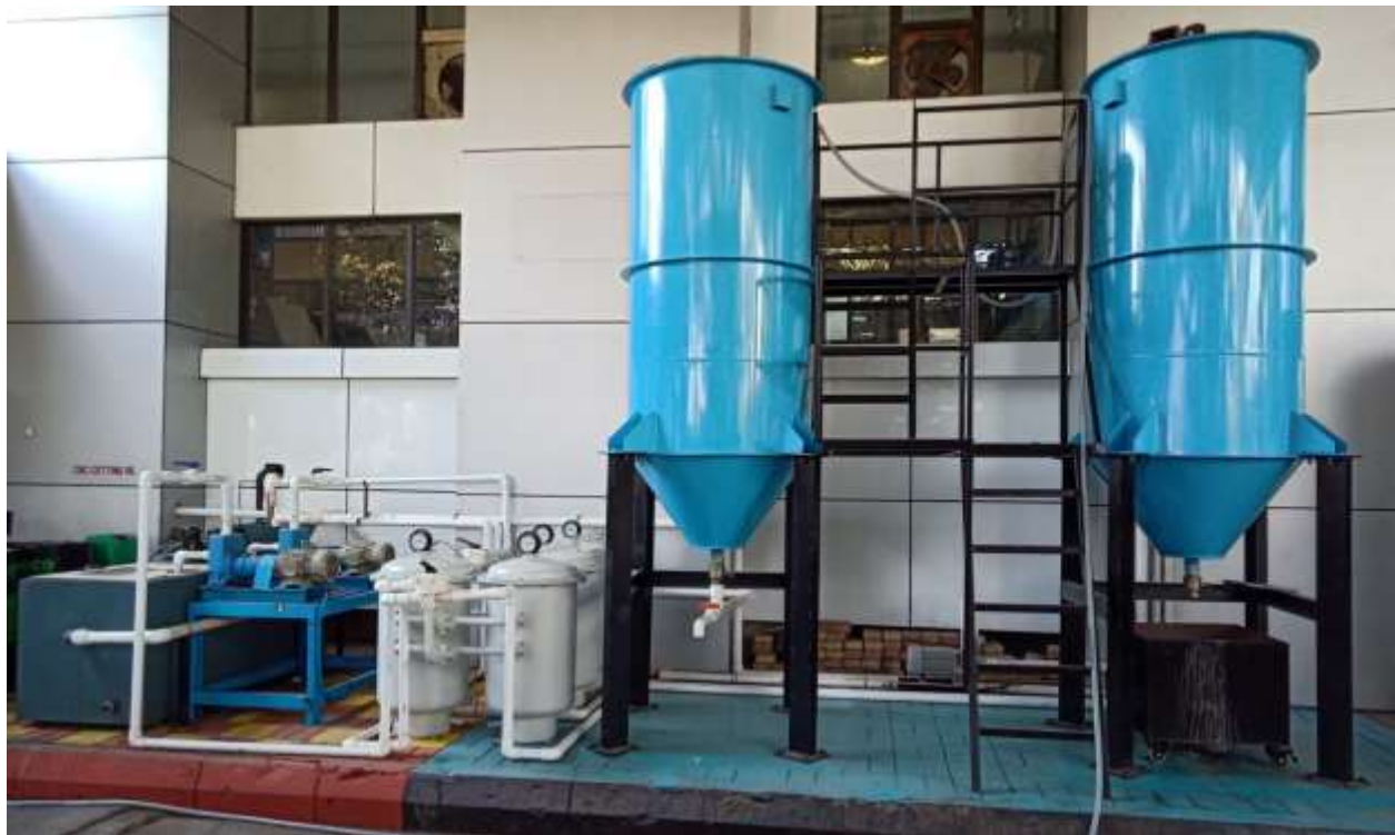
Figure 2: Sand-bed filtration system implemented by Innovation Filter System
