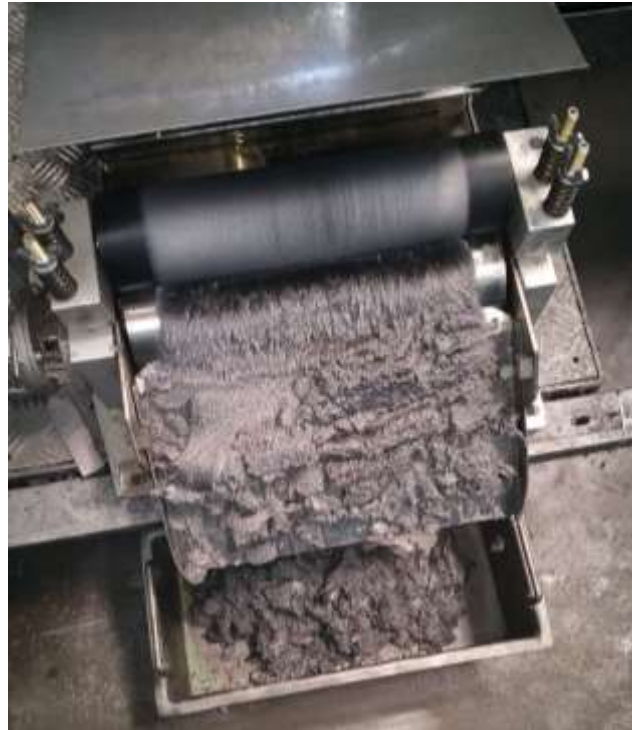
Figure 1 Rare-earth high Gauss magnetic separator for prefiltration to reduce dirt load on main filter elements.
