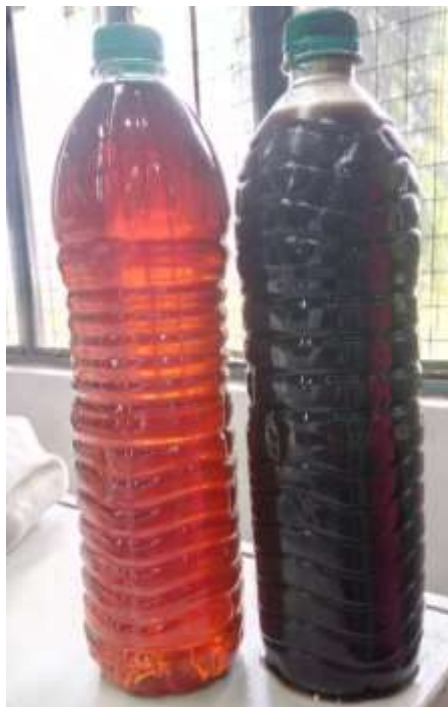
Figure 2 Filtration result on original oi (5 cSt viscosity oil) (l - clean oil, r - dirty oil)
