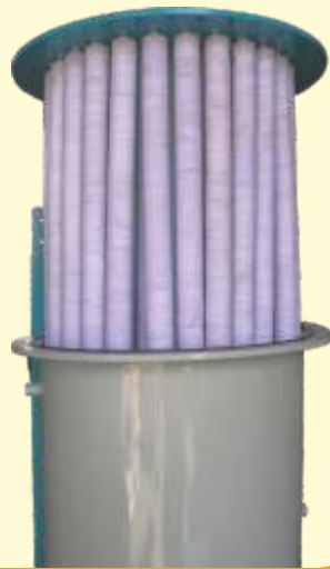
'160 lpm aluminum grinding filtration system at Nirlep Engineering Ltd, Aurangabad'
